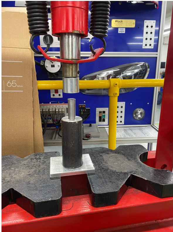
Compression tooling and specimen release. Original report S3 page 22.
